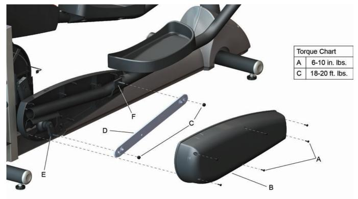
**Tools required:** Phillip #2 magnetic screwdriver, 5mm Allen wrench set, 6mm and 1/2" socket, 1/2" wrench
